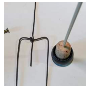
4. Bend the 8" wire into an inverted U shape. Thread the U wire through the loop.
